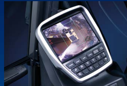
SAVM: secure field of vision in all directions through ten views including 3D bird's eye view and 2D/4CH view.
